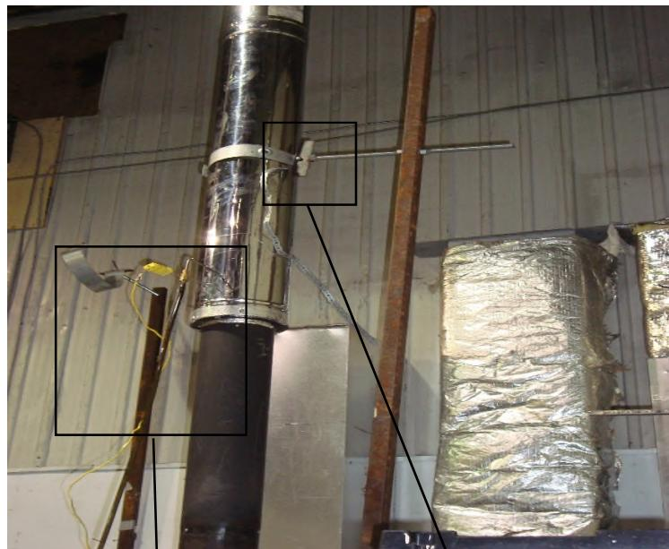
Picture 3.1: Gas analysis and temperature probe
