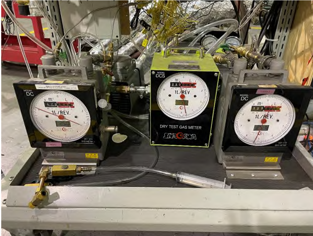
Picture 11: Dry gas meter
